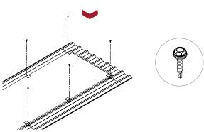
New screws and bonded galvanised washers secure each bracket and panel in place.
