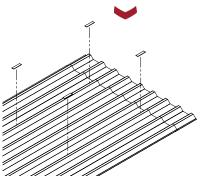
Sealing tape is placed on the roof to help position the panel in place.
