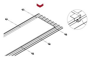
Bespoke fabricated brackets are lined up with existing screw holes.
