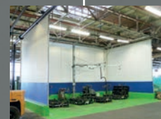
Flexiwall – washdown bay
