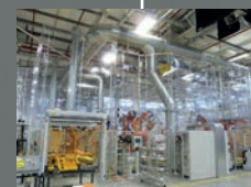
Flexiwall – spark containment/robotic welding enclosure
