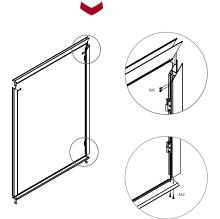
Aluminium frames are bolted together at all four corners. Single doors supplied preassembled. Double doors supplied with self-tapping screws for easy selfassembly on site.
